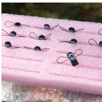
The ‘light-level’ locators (above) track movements between wintering and breeding grounds by calculating the individual’s position using sunrise and sunset times. Each weighs only 0.45 gram.
