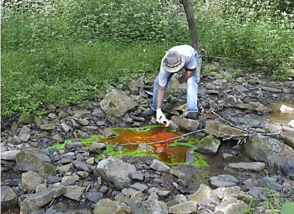
A fluorescent tracer dye is being added to a sinking stream in the Bullpasture River drainage to determine where the water returns to the surface and the travel time for the tracer.
